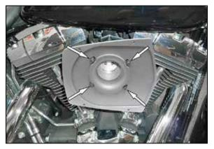
12. Install the provided gasket between the back plate and air filter base using provided hardware. Slightly tighten at this time. Using the air filter cover clock the filter base in position then finish tightening filter base plate.
