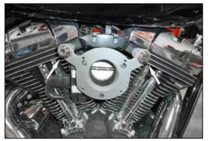
10. Using the two provided crankcase breather bolts install the back plate onto the vehicle as shown. Do not tighten the breather bolts at this time.
