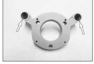
9. Install the remaining two o rings onto the front of the back plate as shown.
