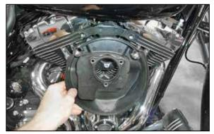
6. Remove the air filter breather base as shown. NOTE: K&N Engineering, Inc. recommends that customers do not discard the factory air intake components.
